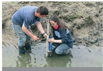
**Figure 2.9:** Installing a sonde (a type of transmitting sensor) to monitor conductivity, depth, salinity and turbidity in an intertidal channel. Photo: Heidi Burgess.
