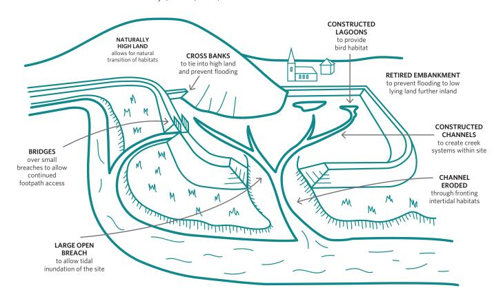
Figure 5.13: Aspects of a theoretical managed realignment project.
