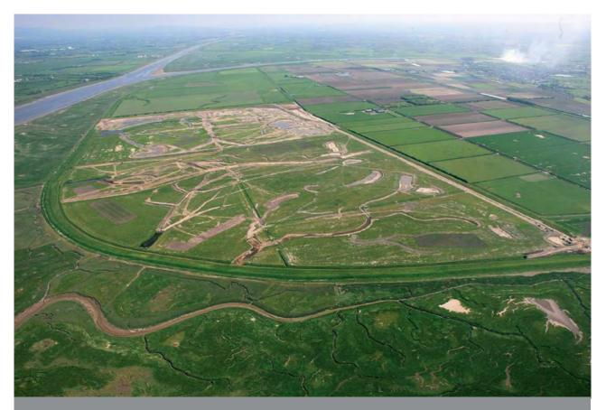
**Figure 5.14:** Hesketh Out Marsh West in the Ribble Estuary during the construction phase. The light brown linear features within the site are channels being excavated along the line of former tidal creeks which existed prior to lanc claim. A number of shallow lagoons can be seen at the head of the creeks. Photo: RSPB.
