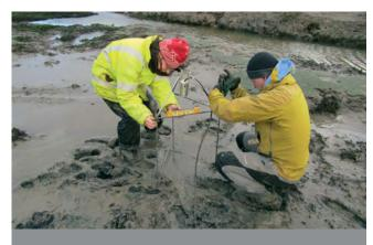
**Figure 2.8:** Installing an ALTUS system (a submersible altimeter), which can measure fluctuations in bed elevation every 15 minutes and can be left in place for several years. Photo: Heidi Burgess.
