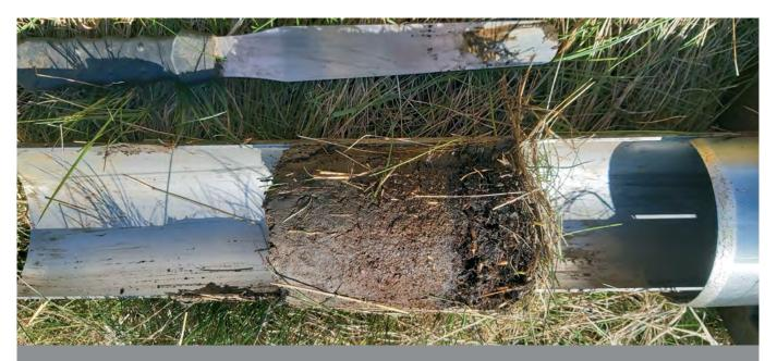
Post-restoration sediment accumulation in an extended golf-hole cutter core (10cm diameter) recovered from RSPB Nigg Bay nature reserve (Cromarty Firth). Marine sands and silts, which accumulated rapidly after the realignment, are overlain by organic-rich saltmarsh soils – highlighting active and ongoing soil carbon burial at this site Nigg Bay was Scotland's first coastal realignment project, implemented in February 2003. Photo: William Austin, May 2021.
