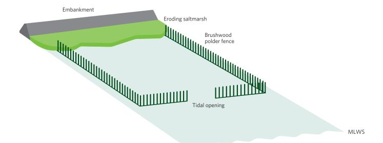
**Figure 5.9:** Basic setup of a single sedimentation field (also referred to as sedimentation polder) consisting of brushwood groynes inserted in the mudflat to form an enclosure with a tidal inlet (adapted from Colenutt, 2001).
