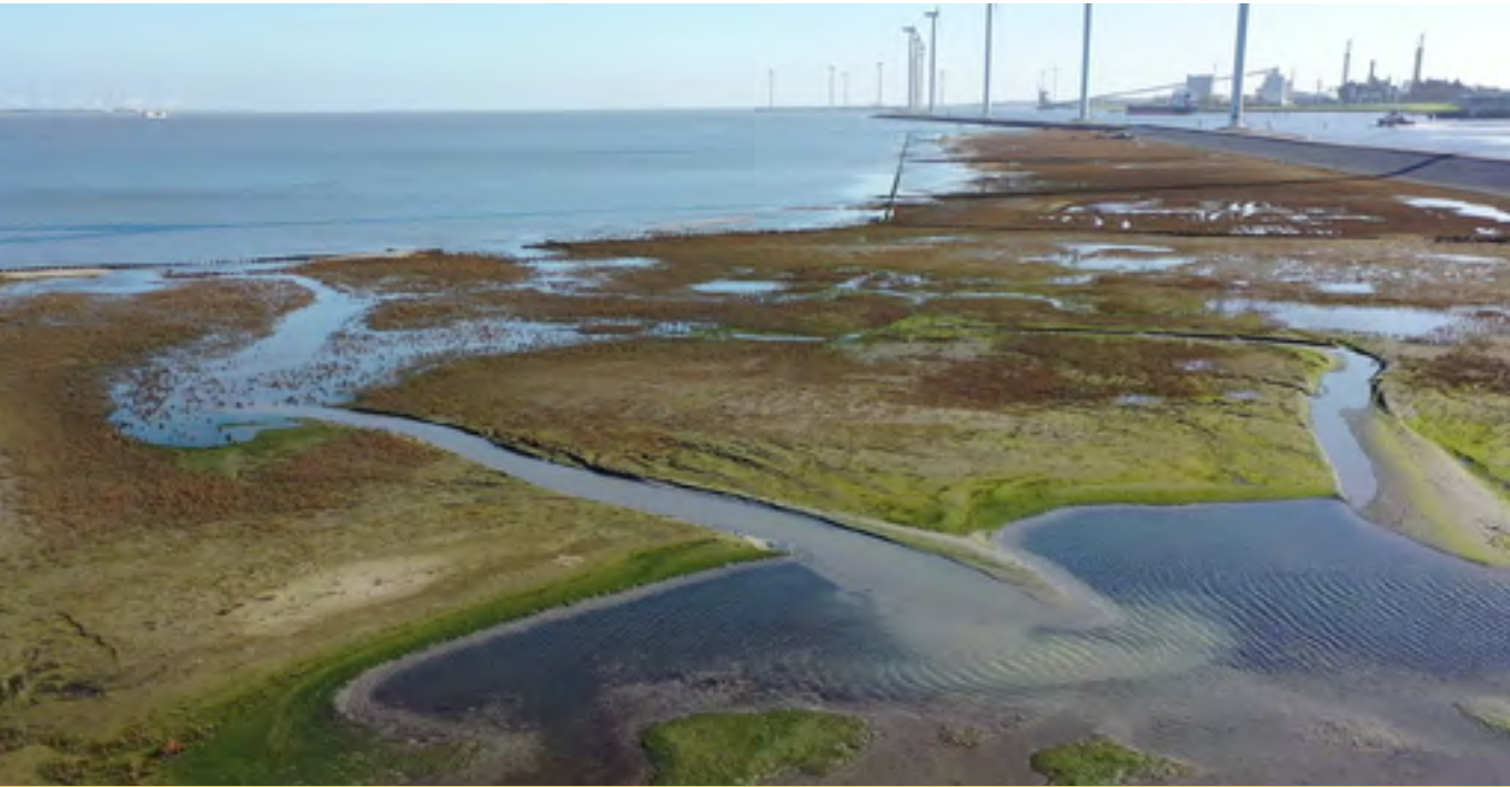
Development of the Marconi Marshes following placement of dredged material arising from the Port of Delfzijl, in the Elms-Dollard estuary, Netherlands, including the experimental use of different compositions of fine sediment (EcoShape).
