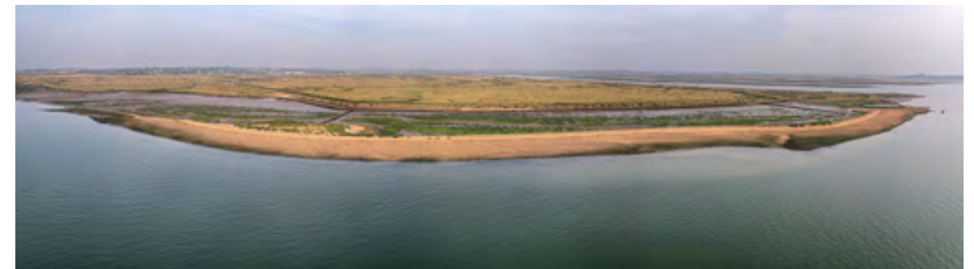
An aerial view of the sand and gravel barrier shown in the image above, located along the eastern seaward face of Tollesbury Wick Reserve. Since placement (1990s), this breakwater feature has facilitated accretion on its leeward side to the extent that saltmarsh vegetation is beginning to colonise the elevated mudflat in front of the defences (Jim Pullen Surveys).
