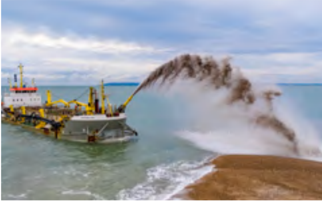
Figure 2.2: Different disposal techniques, from top: Clam shell excavation from hopper (Carol Reid); release of hydraulically pumped sediment via pipeline (Exo Environmental Ltd.); spud barge and hopper barge at marsh transfer and hydraulic pumping station (ABPmer); and coarse sediment rainbow discharge (Boskalis).
